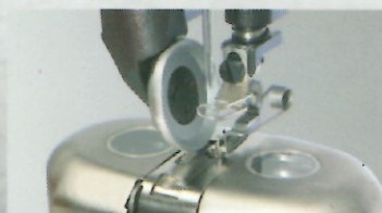
Inspection glass in hook compartment cover for controlling the amount of thread on the bobbin. Easy to change needle plate inserts (from -900/..)
