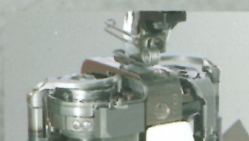
Easily adjustable thread trimmer with reinforced catcher and knife system for short thread ends (up to 15/3 syn.)
