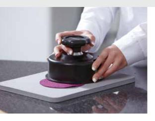
Sample Cutters enable you to cut out rapidly and accurately circular specimens of a fixed diameter.
