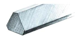
Standard triangular working part cross-section
